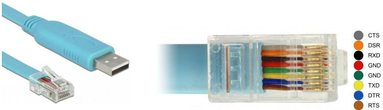
RJ45 Male Pin Mapping (Top View)
